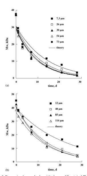
Fig. 3. Decrease in polymer molecular weight of porous, different-sized, PLGA-based microparticles upon exposure to phosphate buffer pH 7.4: (a) lidocaine-loaded systems and (b) drug-free devices (the mean microparticle radii are indicated in the figures). Symbols indicate experimentally determined results, solid curves fitted pseudo-first-order kinetics [Eq. (3)].
