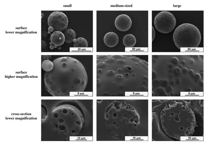
Fig. 1. Morphology of the investigated small, medium-sized and large, lidocaine-loaded, PLGA-based microparticles before exposure to phosphate buffer pH 7.4 (t=0): SEM pictures of surfaces (lower and higher magnification) and cross-sections (lower magnification) (as indicated in the figure).
