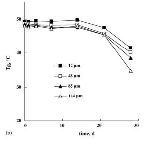
Fig. 5. Changes in the glass transition temperature  $(T_{\rm g})$  of PLGA in different-sized, porous microparticles upon exposure to phosphate buffer pH 7.4: (a) lidocaine-loaded systems and (b) drug-free devices (the mean microparticle radii are indicated in the figures).
