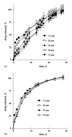
Fig. 2. Effects of the microparticle size on lidocaine release from PLGA-based microparticles in phosphate buffer pH 7.4: (a) porous systems and (b) non-porous devices (the mean microparticle radii are indicated in the figures; please note the different scaling of the *x*-axes).
